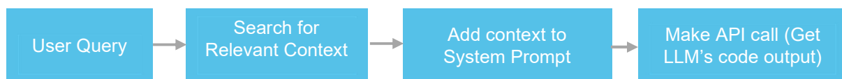
Figure 4 - The flow for implementing a RAG to do data retrieval. Note this is the same as CAG, with the addition of the second ‘Search for Relevant Context’ step.
